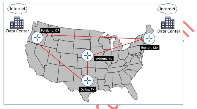
The four hub locations are interconnected in a ring with high-speed 10 Gigabit Ethernet Metro-E circuits from various service providers. These core routers form the OSPF are 0 backbone today. These hub locations also serve large distribution site with approximately 400 employees per location. A 24-hour call center runs across these four locations as well. Internet services are provided to all locations via the Boston and Portland distribution centers.
